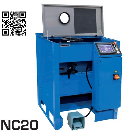
Finn-Power NC-machines have proven to be the most reliable and widely used nut crimping machines in the industry. NC-machines provide fast and accurate crimping for fitting manufacturing.
