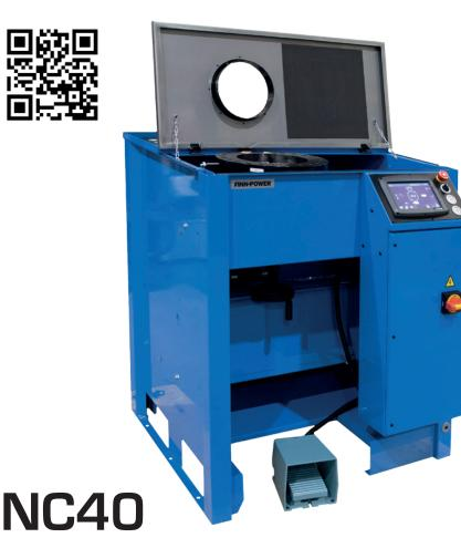
Finn-Power NC-machines have proven to be the most reliable and widely used nut crimping machines in the industry. NC-machines provide fast and accurate crimping for fitting manufacturing.
