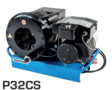
CS-models have been designed for service van use. Also available as Z-model with separate hydraulic unit for better weight balancing and space usage in service van. CS machines are battery powered with 12V or 24V crimping head on left as standard. Right versions available as option.
